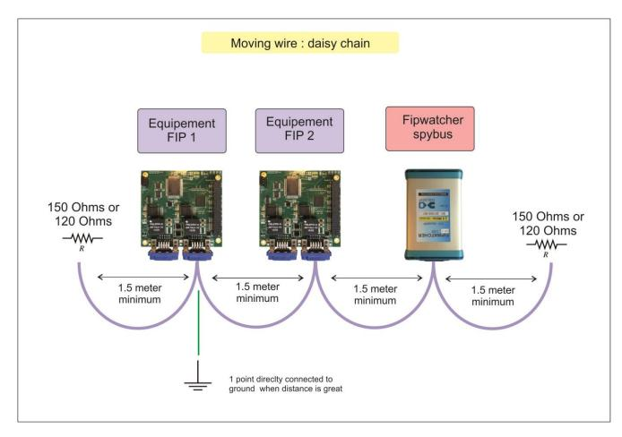
Note: you can use 1 d-sub on our EXOLIGENT card, left or right whatever but only one, the second one is use for redundant network. D-sub are not connected together, it is two independent FIP lines.
