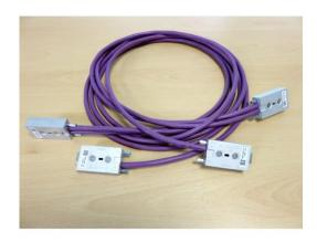
FIP cable test/dev 4 points daisy chain 4 point. Ref 203-600 For installation/tests use **only** compatible FIP cable 150 Ohms or 120 ohms, otherwise the network will generate errors frames or alterated performances.
