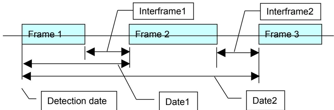
Figure 31: Time measurement and displaying principle
