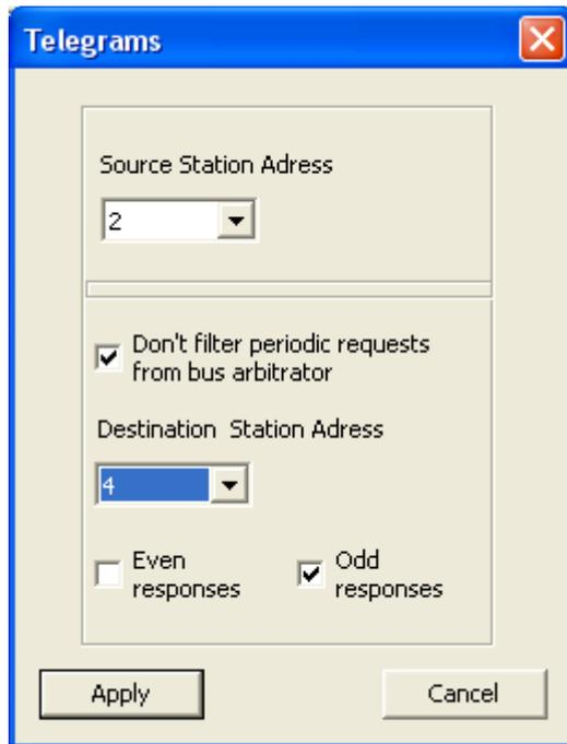
Figure 41 : Dialog box "Telegram Frame Definition"
