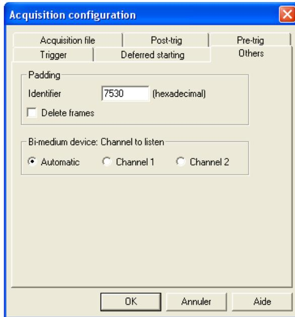
Figure 11: Acquisition configuration –Others tab
