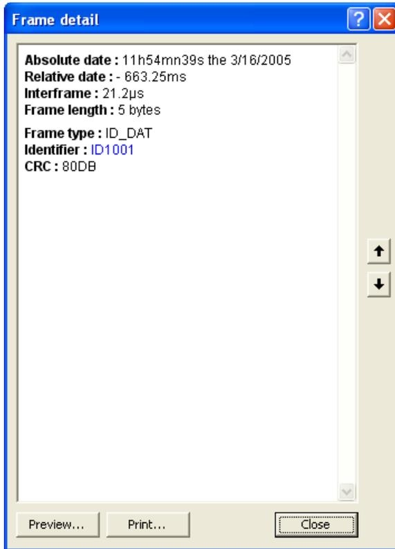
Figure 51: Result of the detail of an "ID\_DAT" frame according to the example file
