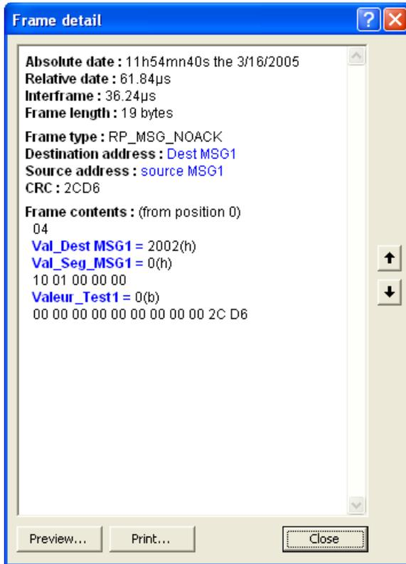
Figure 53: Result of the detail of an "RP\_MSG" frame according to the example file
