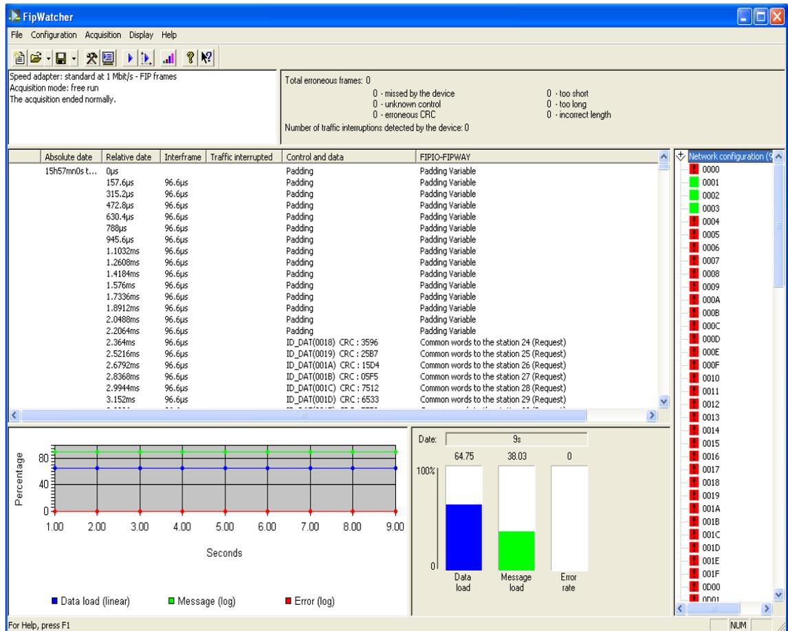
Figure 47 : Compute the data rate with defined FipIO padding frames.
