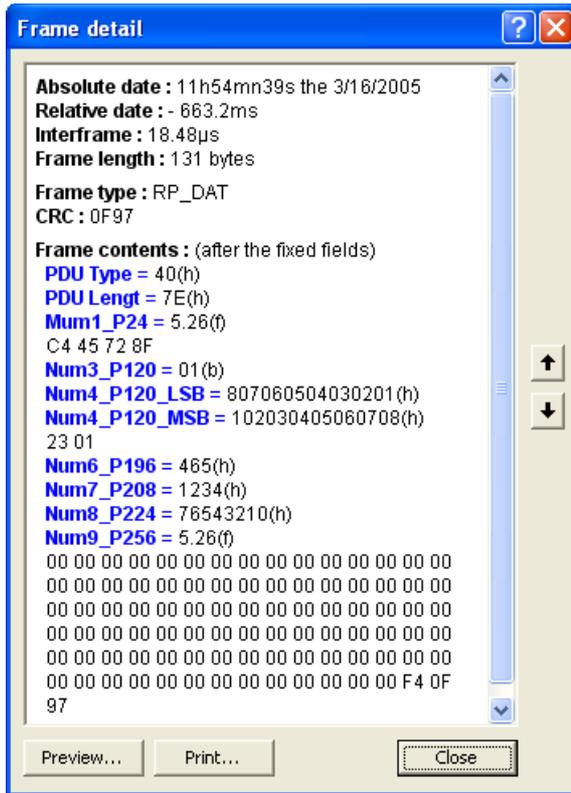
Figure 52: Result of the detail of an "RP\_DAT" frame according to the example file
