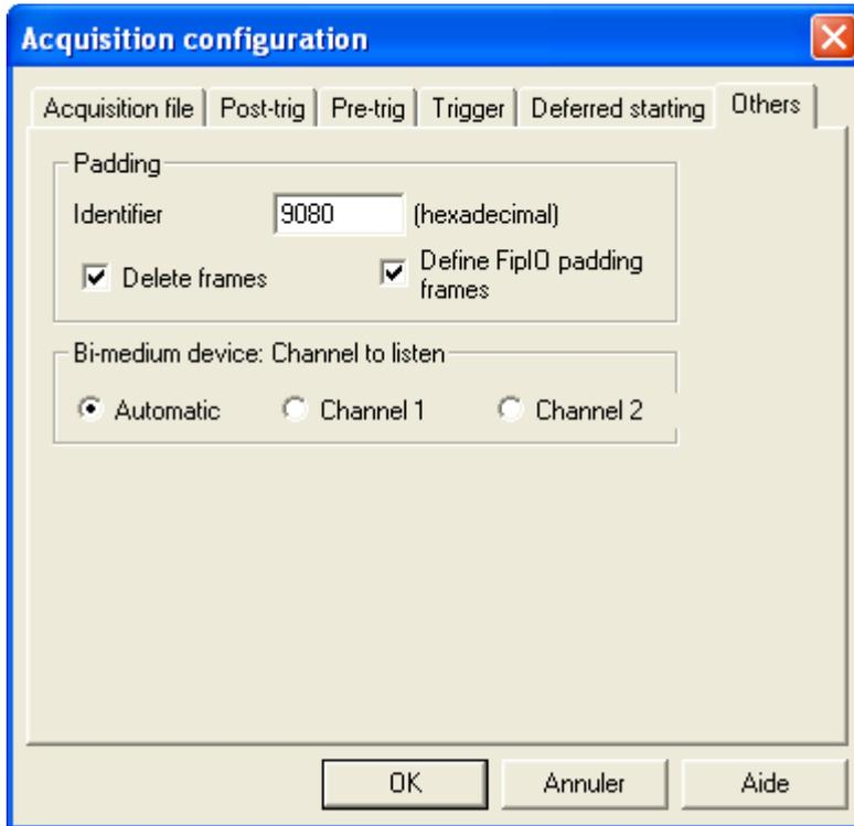
Figure 46 : Eliminate the FipIO padding frames
