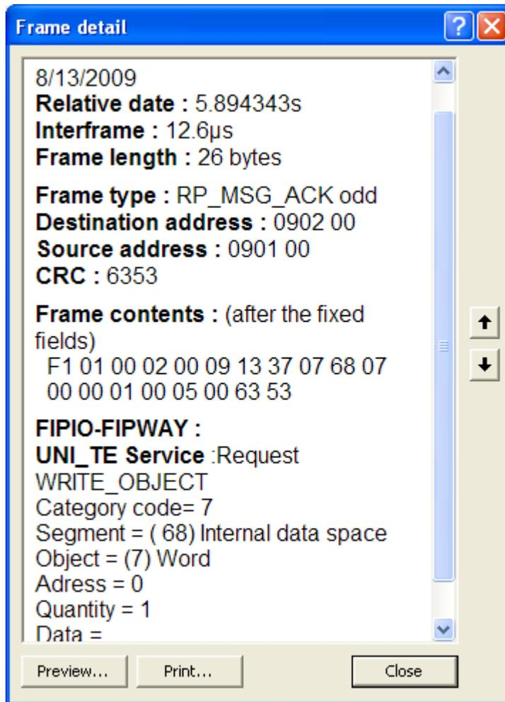
Figure 49 : Detail of a FipIO/0FipWay frame
